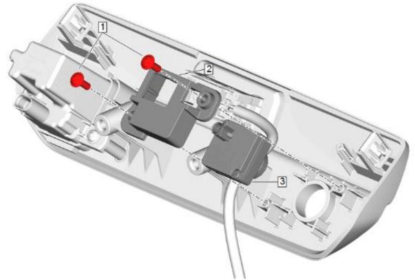
Reverse the above procedures with your new camera module. Make sure to test the new camera module before full reassembly by attaching it to the Coax cable and checking function on the radio. If all is well (which it should be) reassemble and enjoy!
