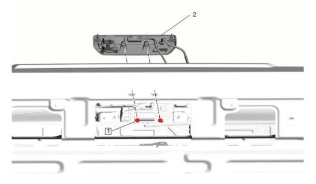
Next remove the factory camera retention bracket and then remove the camera assembly.
