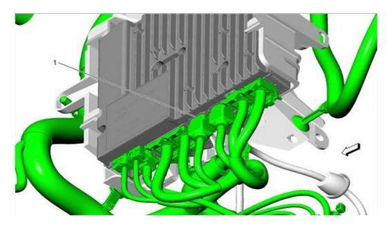
Step 3. Remove the Radio Module by depressing the two retaining clips and sliding the radio module out of the vehicle.
